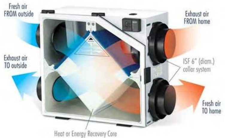
ERV Energy Recovery Ventilation System
